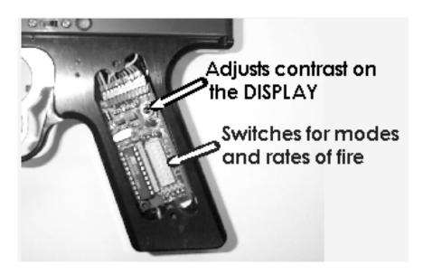
Mode selection is accomplished using switches 1 thru 3. The following configurations will give you the desired modes.
